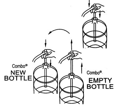
Do not place suction wand on floor, counter, or sink as this could contaminate the suction wand assembly. If bottle is over filled, dispense enough water to allow the suction wand to be pushed to bottom of bottle.
