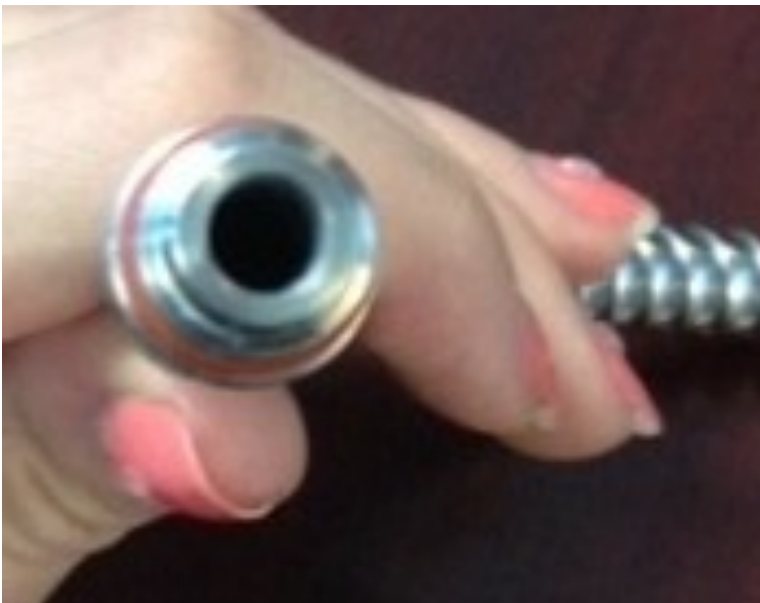
Flex Hose Normally attached to Top Spout No mineral buildup (Front View)
