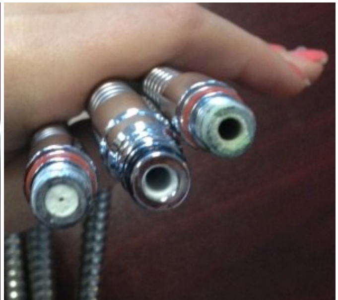
Flex Hose Three Examples With mineral buildup
