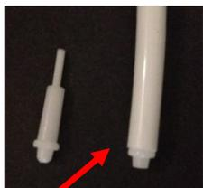
Flow Restrictor inserted in 1/4" tubing
